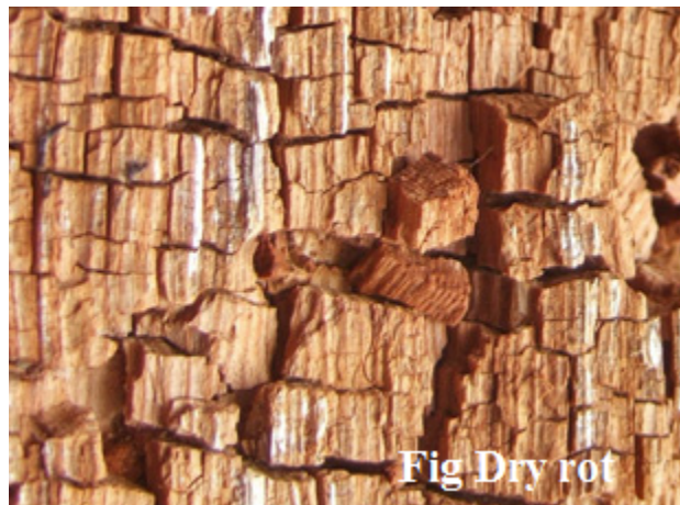
Fig. 10: Figure 7-10. Dry rot defect in wood
