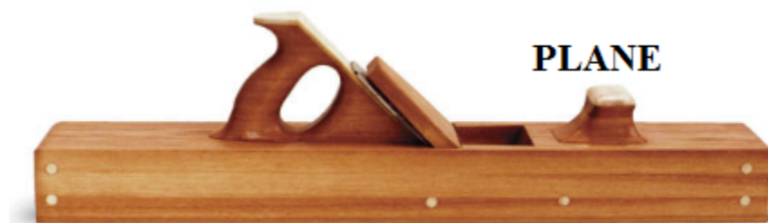
Fig. 2: Figure 5-2. Plane used for shaving and shaping woods
